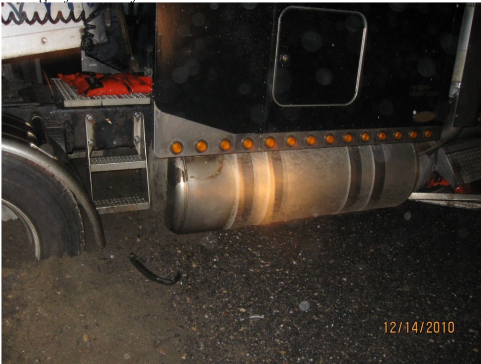
Damaged fuel tank after motor vehicle accident
